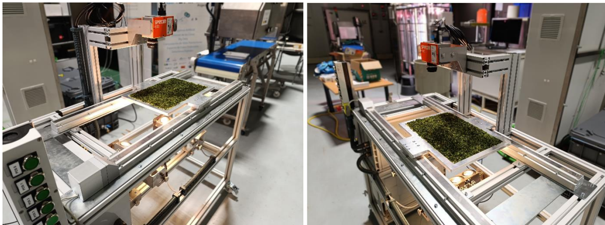
Figure 11: Algae spectral data acquisition with transmittance setup
